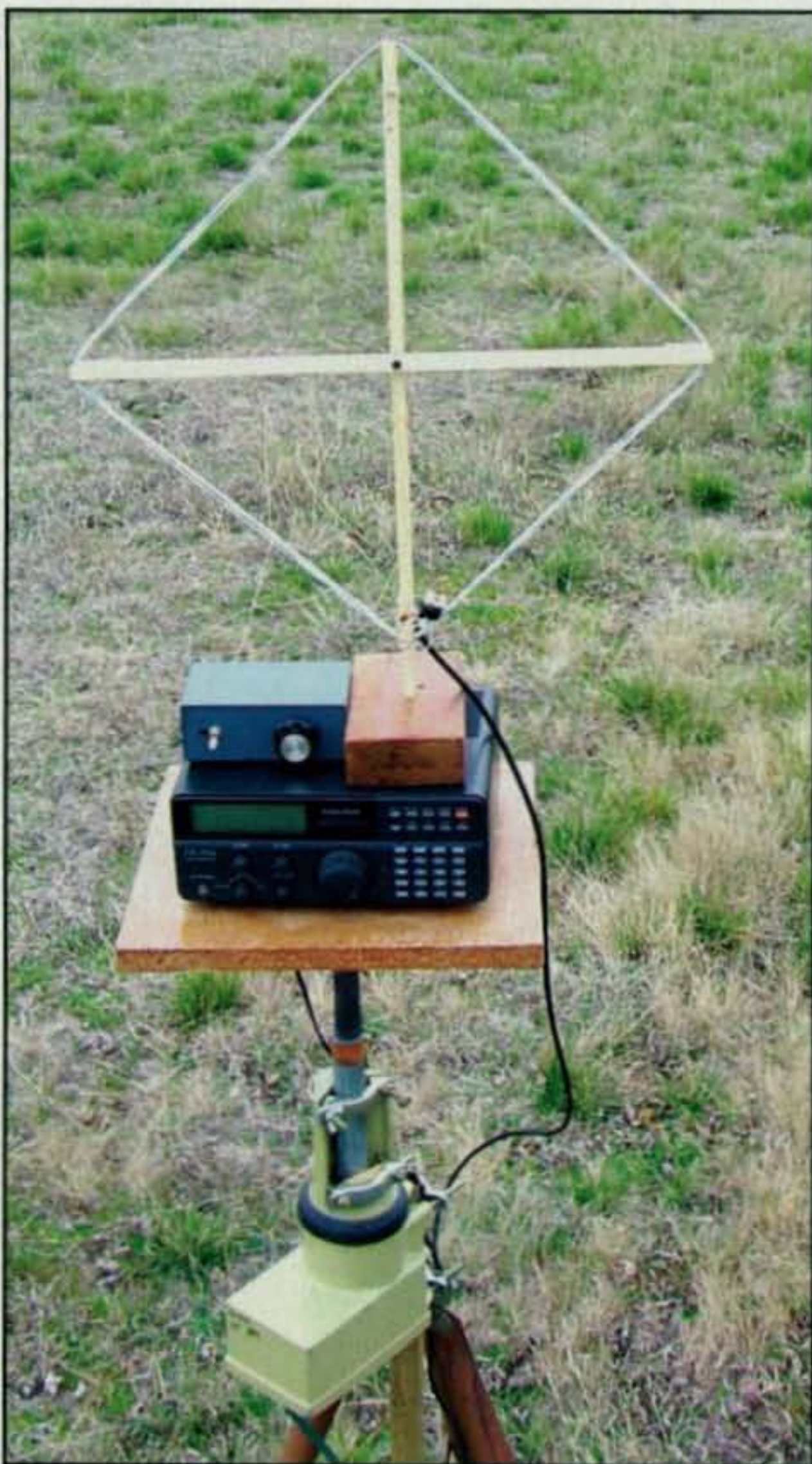
Photo A— The loop antenna and the diode bias supply.
